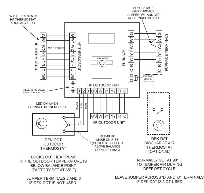
NOTE: IF THE HEAT PUMP THERMOSTAT HAS A SEPARATE EMERGENCY HEAT TERMINAL, JUMPER THE EMERGENCY HEAT TERMINAL AND THE AUXILIARY HEAT TERMINAL AT THE THERMOSTAT.
